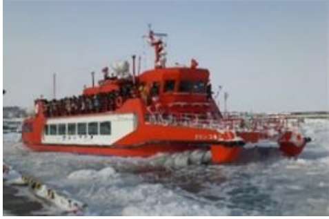
Fig. 6 Sightseeing icebreaker Garinko II with Archimedes' screws. Its prototype was developed for the oil development in Sakhalin.
